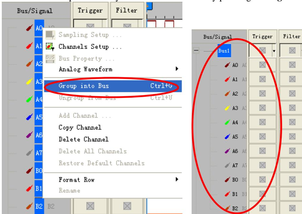
**STEP 2.** Select **Bus1**, and press **Right Key** on the mouse to list the menu, then press **Bus Property** or **Bus bar** on the toolbar to open **Bus Property** dialog box.
