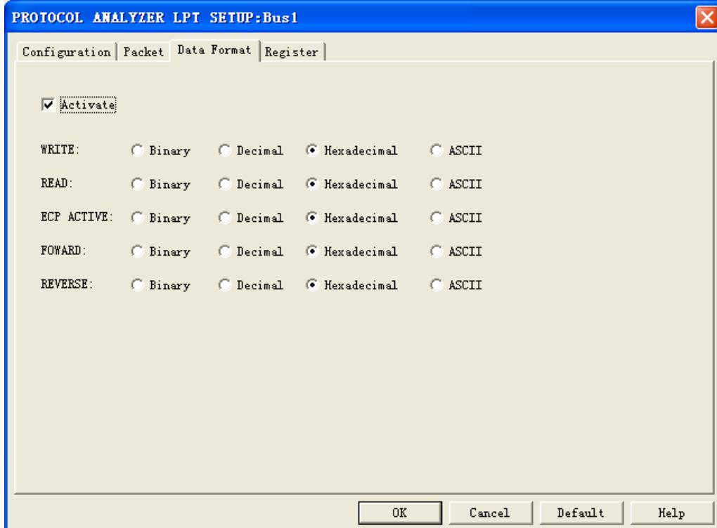
Users can set the Data Format of the WRITE, READ, ECP ACTIVE, FORWARD and REVERSE as their requirements. When selecting the option, Activate, the data formats are decided by the settings in the Module; when not selecting the option, Activate, the data formats are decided by the settings in the main program.
