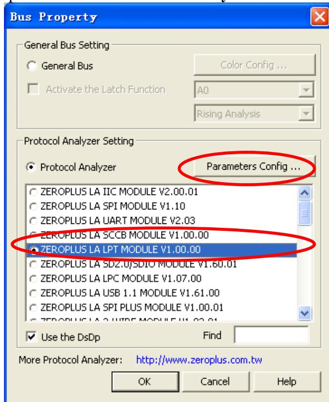
**STEP 6.** Set the Pin Assignment in the Configuration dialog box.
