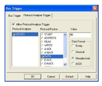
When we enable the Protocol Analyzer 'Trigger' function for the Protocol Analyzer I2C for example, Protocol Packets such as START, ADDRESS, READ, WRITE, A-ACK, D-ACK, D-NACK, A-NACK, ERROR and STOP can be selected to 'trigger' on. The Data Value of the Protocol Packet can be entered according to your requirements.
