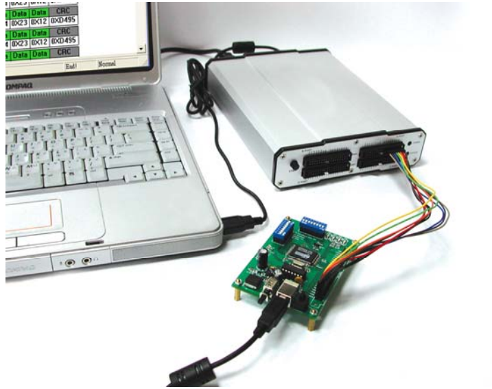
Fig. 2-6: An Assembly of Laptop, Logic Analyzer and a Testing Board
